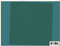
Ca corrosion device after 616 hours under 40°C/90%RH (Thickness of barrier layer: 720nm)
