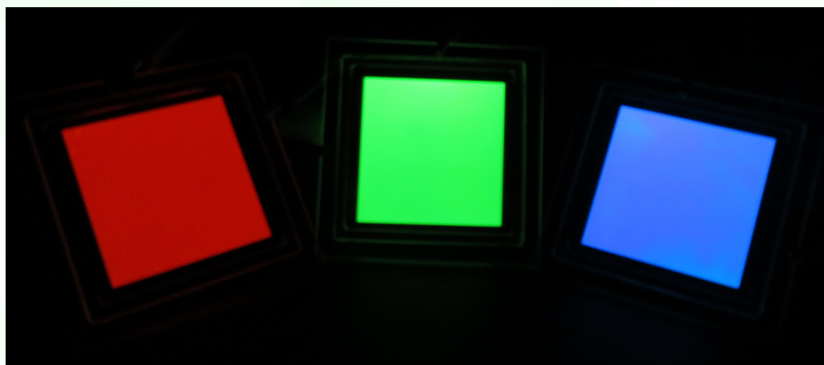
OLED devices fabricated using spray coating
