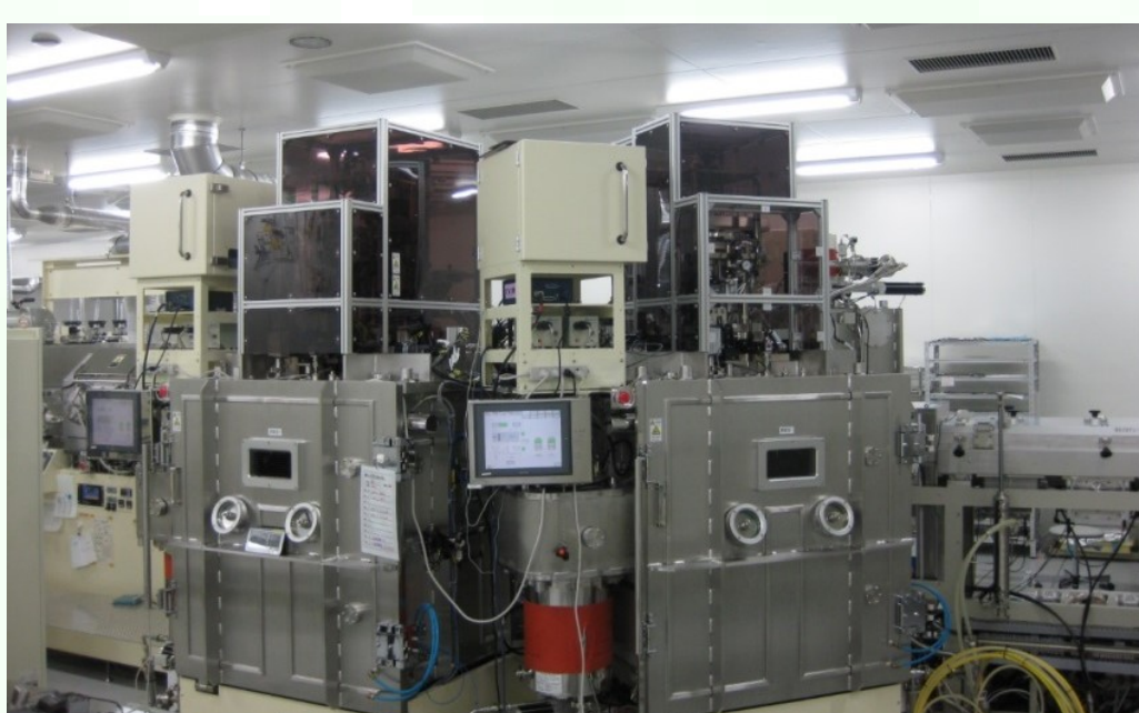
OLED vacuum evaporation equipment "ELVESS" (Tokki)
