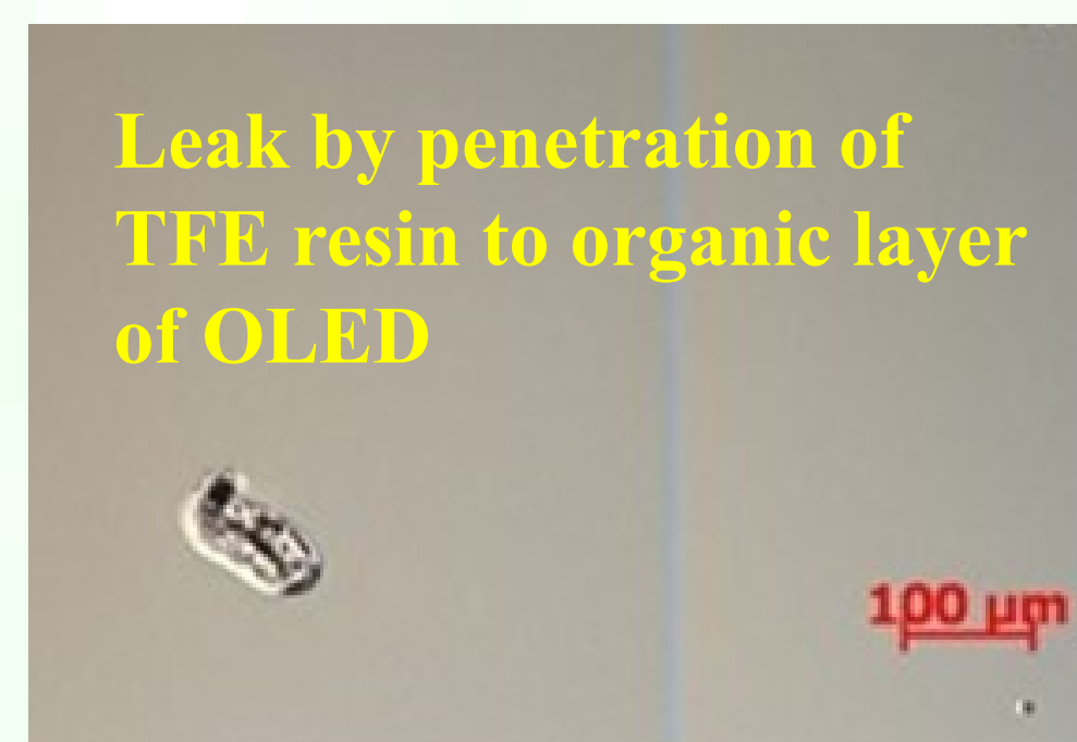
b) Observation of leak point by confocal microscopy
