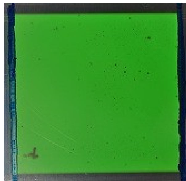
Panel size: 50mm x 50mm Emission area: 32mm x 32mm
