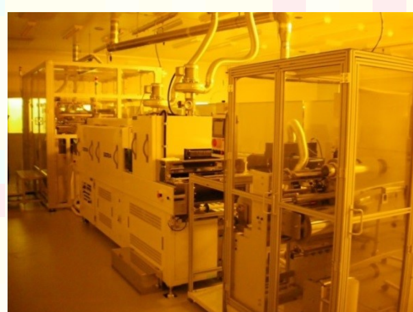
R2R screen printing and slit-coating (SERIA)
