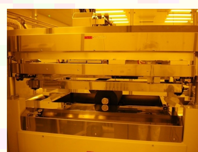
Gap-less screen printing equipment (SERIA ENGINEERING)
