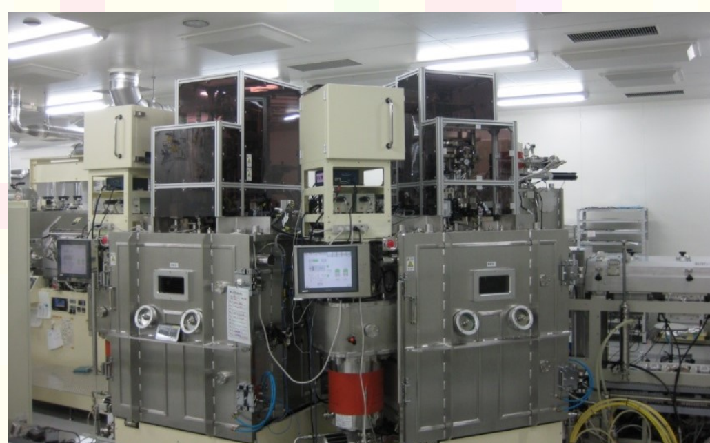
OLED vacuum evaporation equipment "ELVESS" (Tokki)
