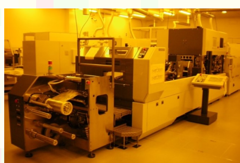
R2R gravure offset and flexography printing (Komori Machinery / Taiyo Kikai)
